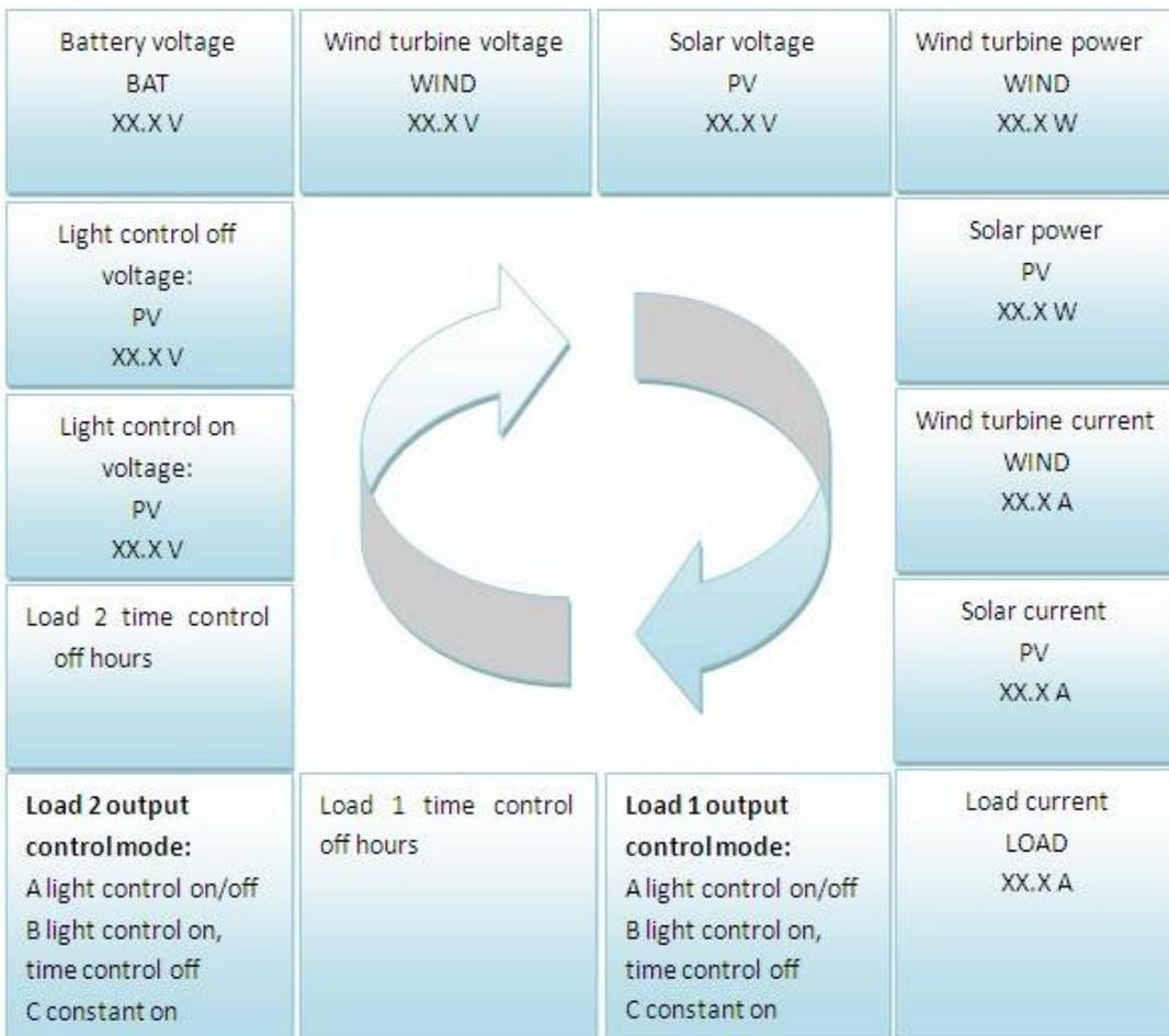
LCD can display three output control modes as follows:
